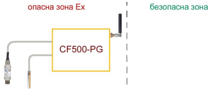
CF500 with installed GSM board and external antenna
